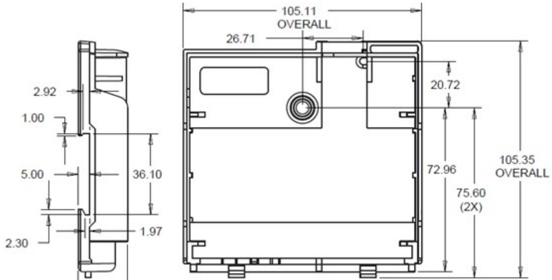
**Figure 2 - Mk10H Mounting Dimensions**
