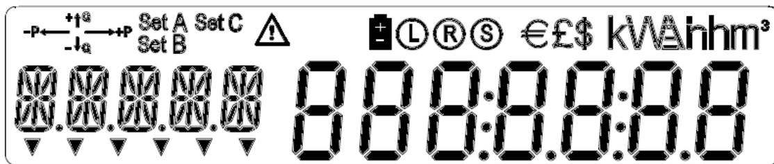
Figure 6 - LCD with all Segments ON
